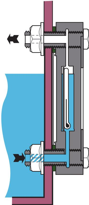
Three sizes in each range are available on the same basic design with the hollow mounting bolts to allow fluid to enter and register on the inside of the lens.
