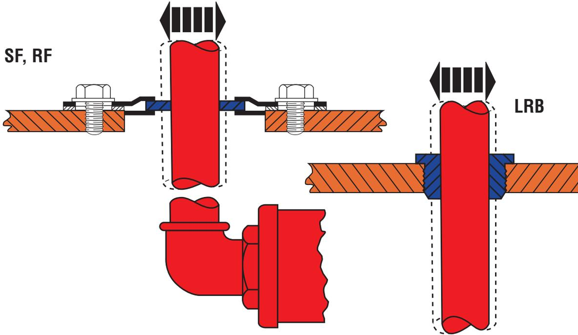
**Lenz SF Suction Flanges, RF Return Flanges, and Return Bushings are designed to seal pipes where they pass through the reservoir top plate.**
