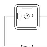
The electrical sensor is stamped N/A (normally closed) or N/O (normally open) and also marked 60°C (148°F) or 70°C (158°F) for switching temperature.
