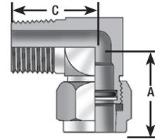
**400-L • Long Male Elbow***Part Numbers Include body nuts, sleeves, "O-Rings" and Back-Up Washers.*
