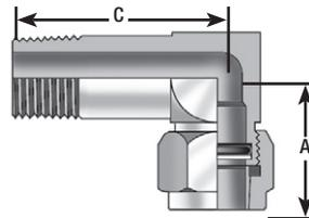
**400-LL • Extra Long Male Elbow***Part Numbers Include body nuts, sleeves, "O-Rings" and Back-Up Washers.*
